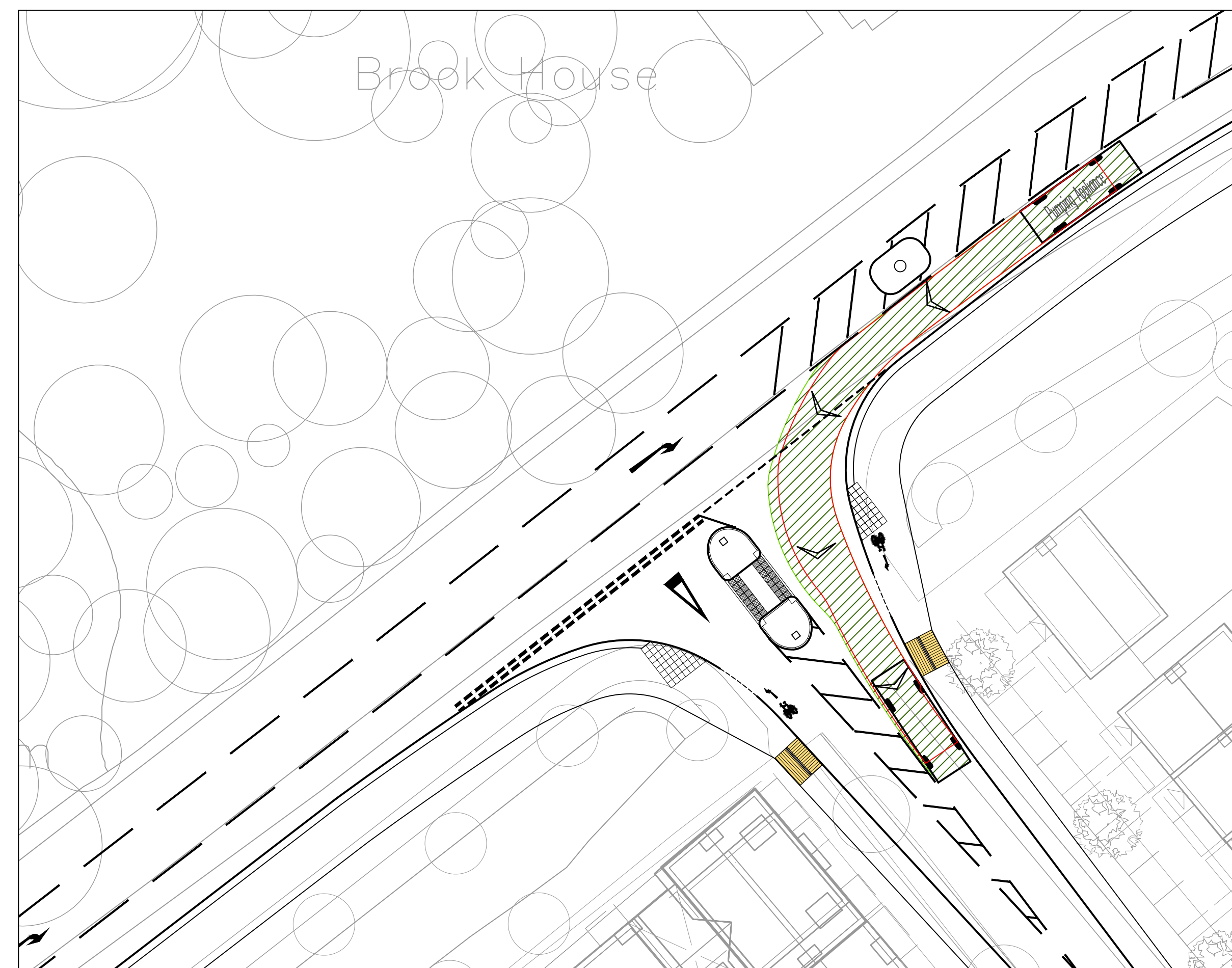
7.9m EMERGENCY VEHICLE INBOUND FROM THE EAST
