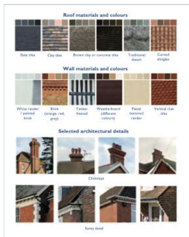
Above: The Code identifies common building materials, colours and details found in Hailsham, and which should inform the choice of materials and architectural features in new development.
