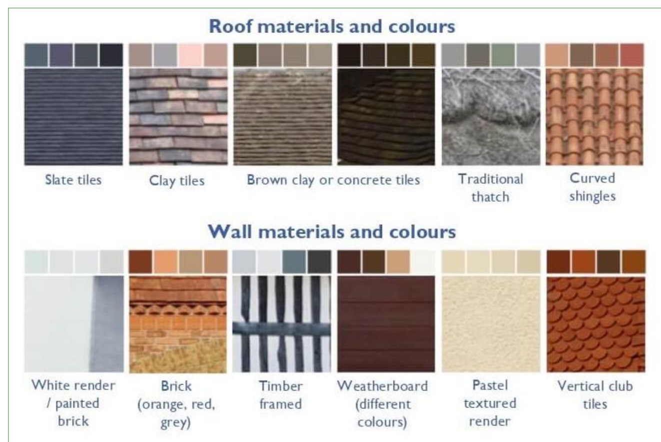
Figure 55: Common materials and colours found on buildings in Hailsham and which can be combined to create variety and interest in new development
