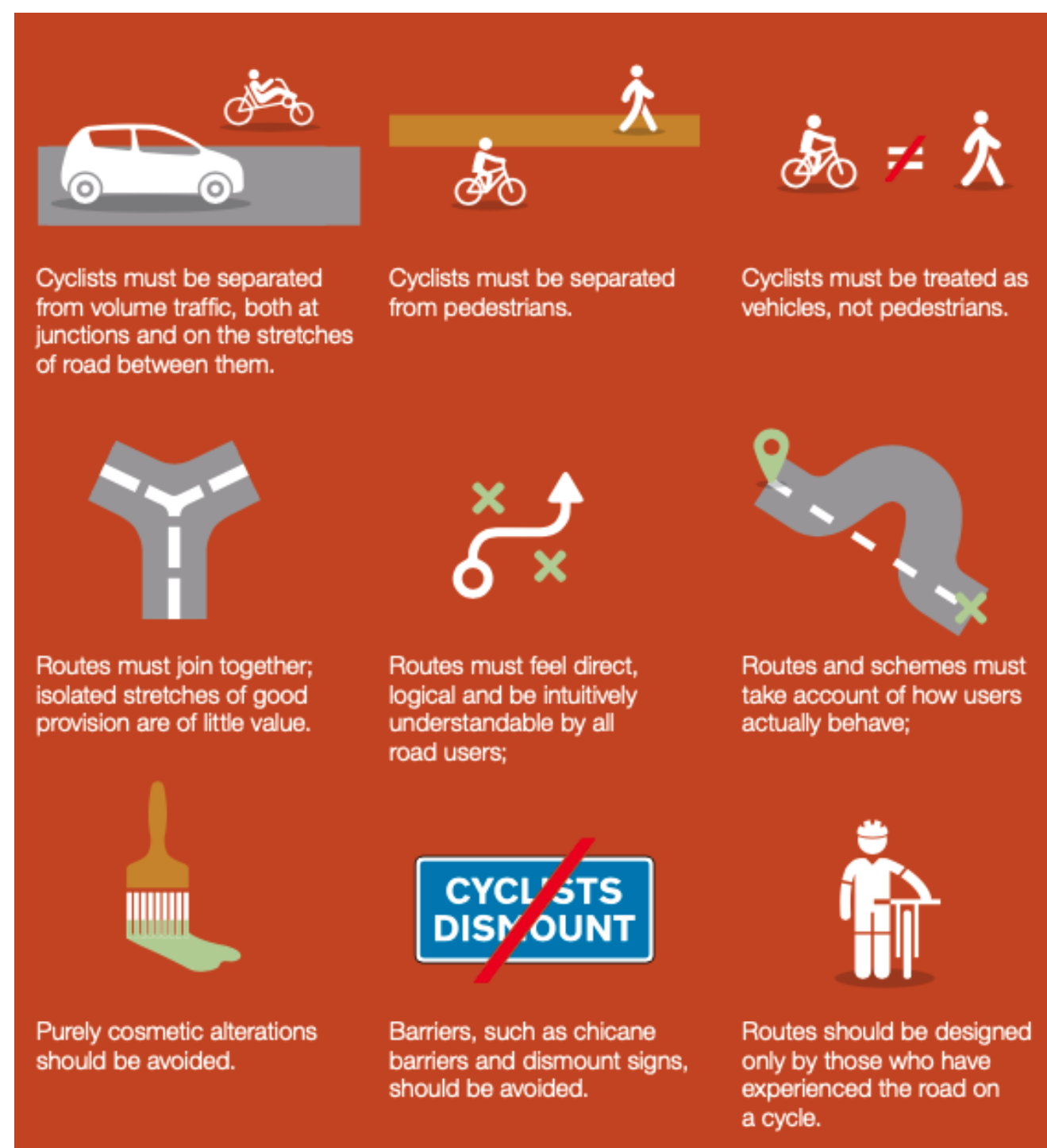
Figure 81: Key design principle for cycling (source: DfT, 2020, Gear for Change)
