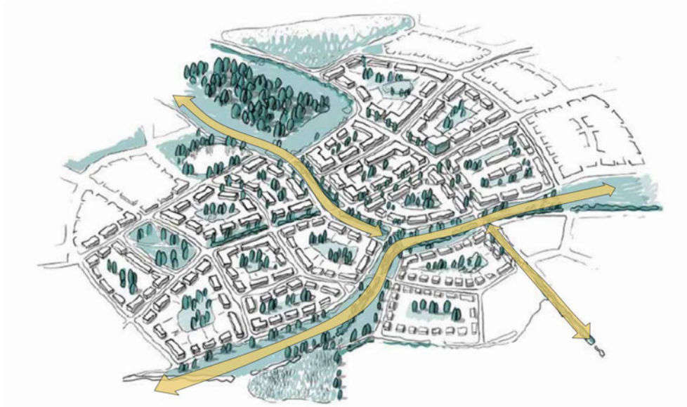
An illustrative diagram from the National Model Design Code (NMDC) showing (in principle) how green corridors can be designed into developments.
