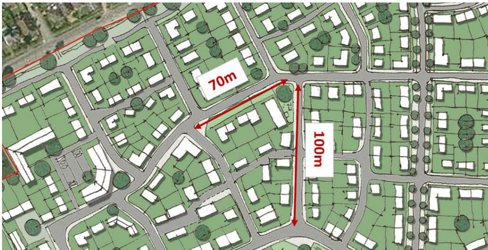
Examples of a well-connected layout with block lengths between 50m & 100m.
