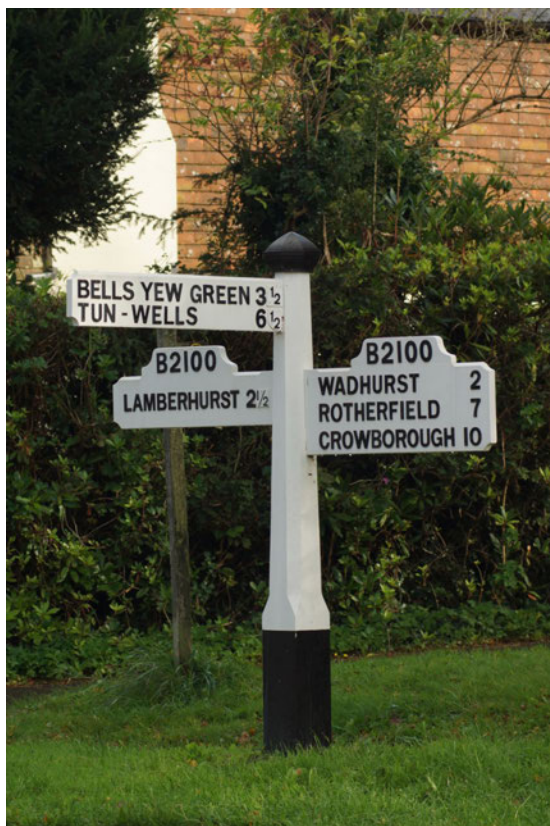
Traditional East Sussex Fingerpost with cast metal cap and oak post.
