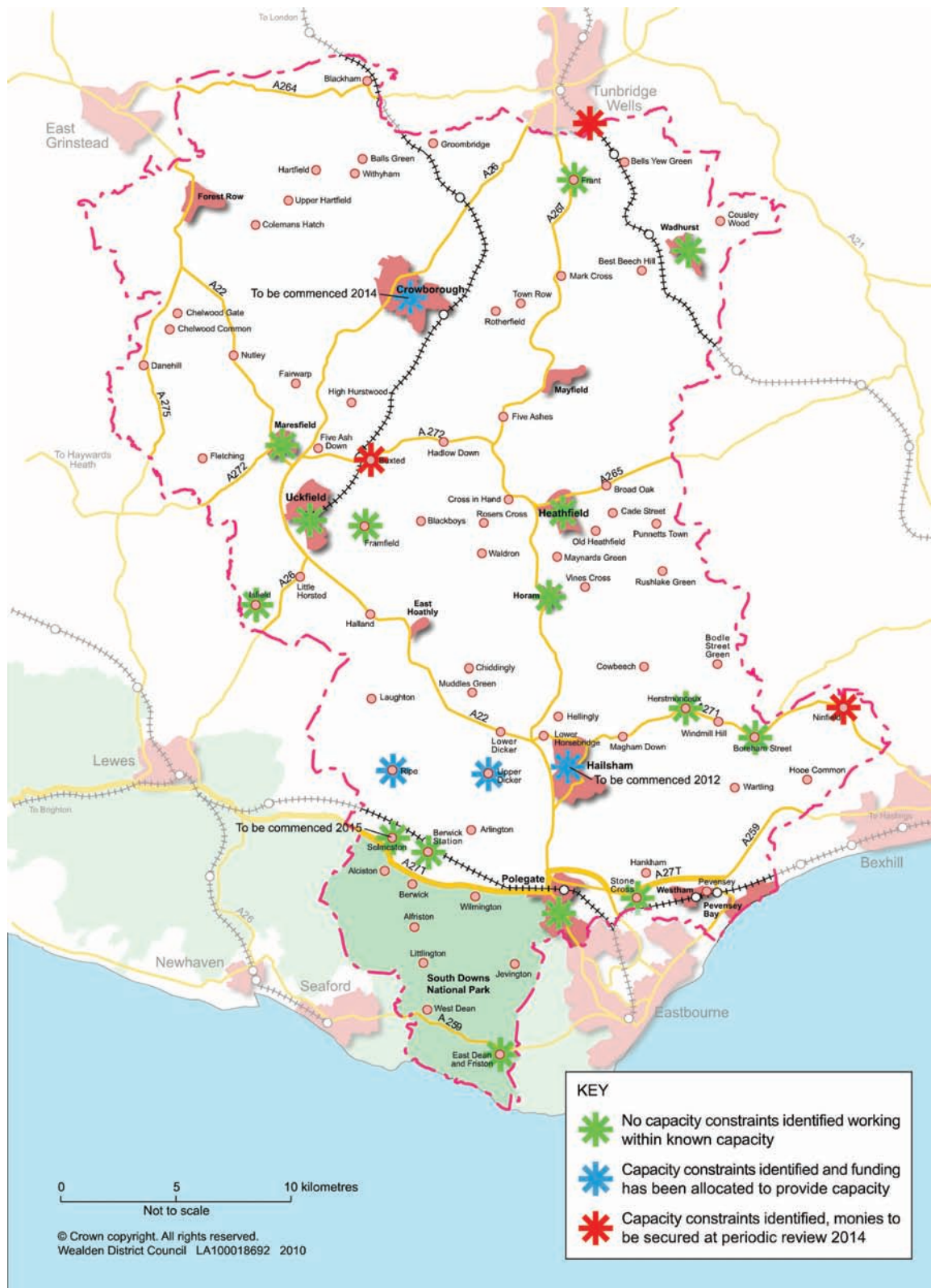
Figure 4 Diagram showing Status of waste water Infrastructure in relation to proposed growth in Wealden
