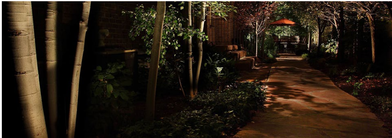
Figure 129: Example of down lighting which was used to illuminate the pathway.
