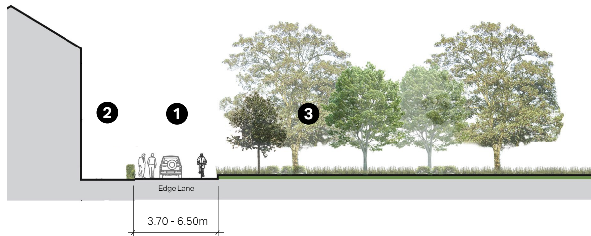
Figure 150: Cross-section to illustrate some guidelines for edge lanes.
