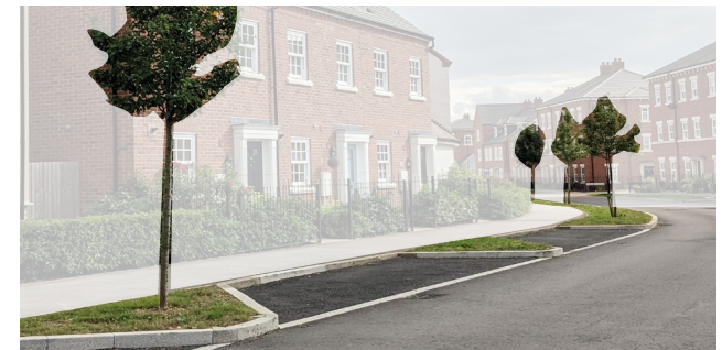
Figure 55: Example of on-street parking bays that are placed between green verges and street trees, elsewhere in UK.
