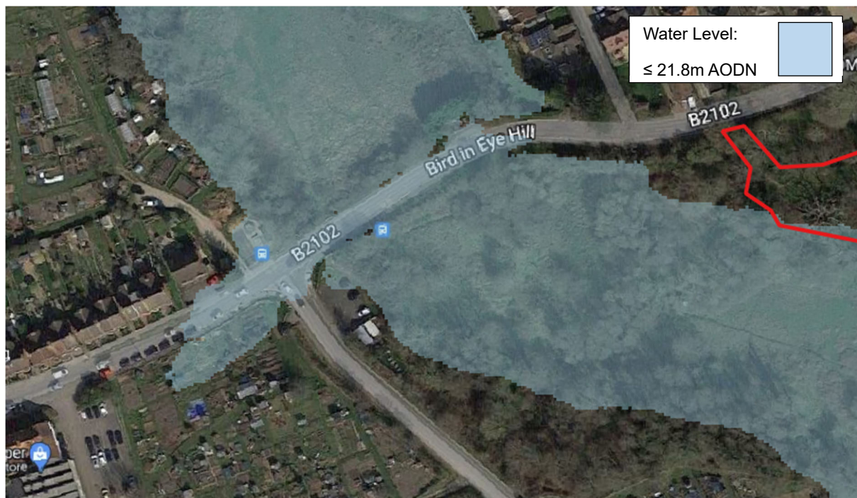
Figure 7 - Flood contour with maximum water level up to 21.8m AODN shown in blue to replicate the extent of flooding witnessed in November 2022 (Imagery ©2023 Google).
