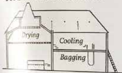
Fig 5.3 Type 2, inset kiln with small conical roof. Cross section.
